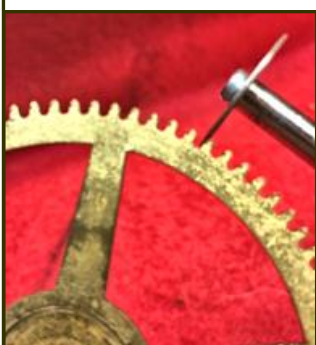
Fig. 5: Reshaping the teeth with a rotary tool
