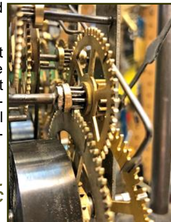
Fig. 6: The repaired wheel in place and the clock running like new!
