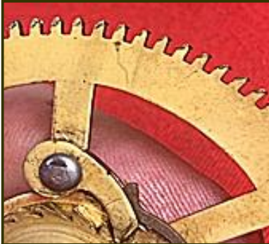
Fig. 1: The damaged teeth on the strike side main wheel
