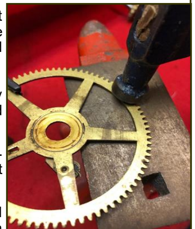
Fig. 4: Flattening and elongating the teeth with a light hammer
